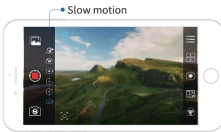
1.Slide the screen, or tickle down the multi-function composite 3-position zoom control switch, and switch the shooting mode to the slow motion mode;
