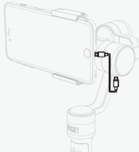
Use Rigiet to phone charging cablee, as shown in the Figure above, with one port inserted into Rigiet to phone charging micro USB output port and another end inserted into the charging port of the phone.
