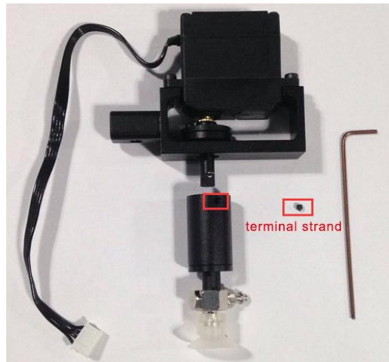
Figure 5.9 Dismantle the suction cup
