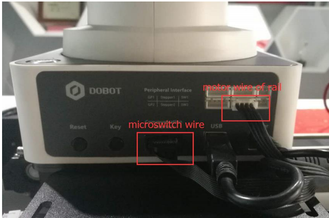
Figure 16.1 LinearRail connect to Dobot arm
