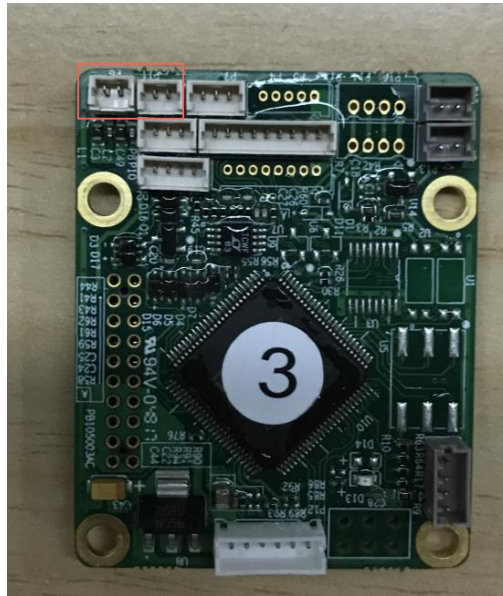
Figure 7.15 Battery interfaces on the Driver Board
