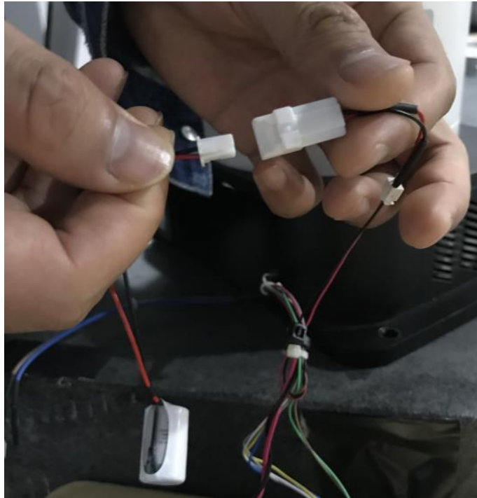
Figure 7.9 Disconnect the connector of the battery from the battery adaptor cable
