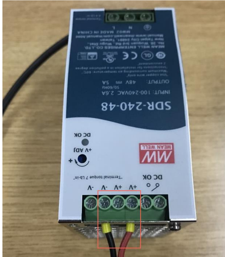
Figure 5.6 Connect power supply output cable to power adapter
