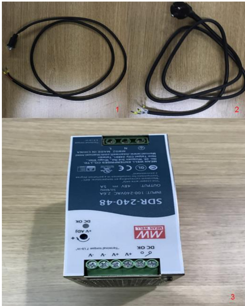
Figure 5.4 Power cables and power adapter
