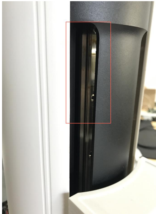
Figure 7.2 Guide rail of Z-axis
