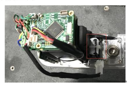
Figure 7.17 Put battery into battery holder
