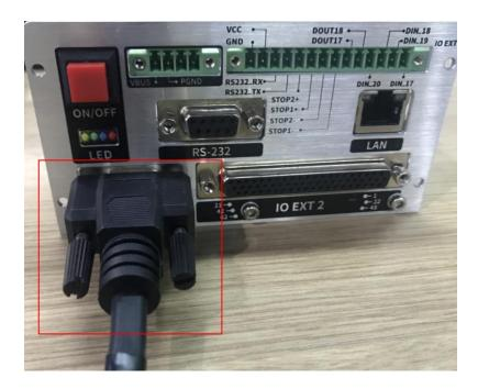
Figure 5.7 Connect to Dobot M1
