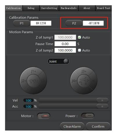
Figure 7.24 Calibration as lefty hand orientation
