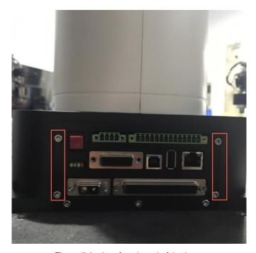
Figure 7.6 Interface board of the base
