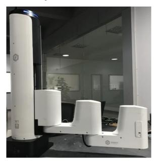
Figure 7.19 Location of Dobot M1 after Factory calibration
