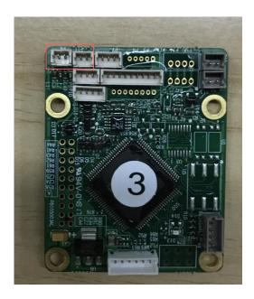
Figure 7.14 Battery interfaces on the Driver Board
