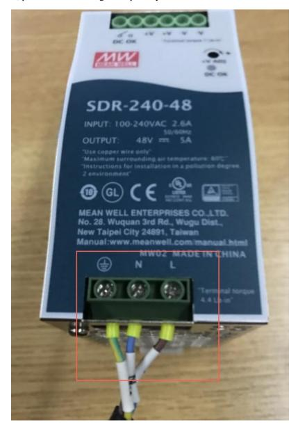
Figure 5.5 Connect power supply input cable to power adapter
