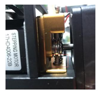
Figure 3.8 Push down the filament (2)
