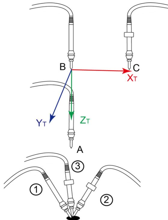
Figure 3.5 Three points calibration method (TCP+ZX)
