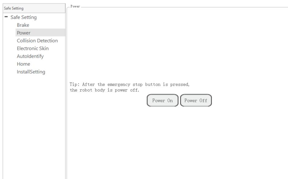
Figure 3.20 Control robot power on and off
