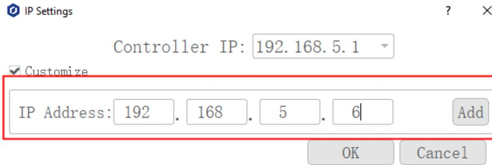
Figure 2.3 Add controller's IP address
