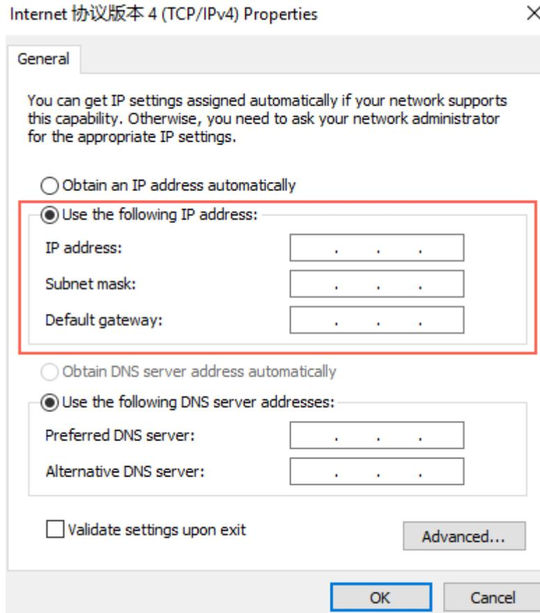
Figure 2.1 IP address modification
