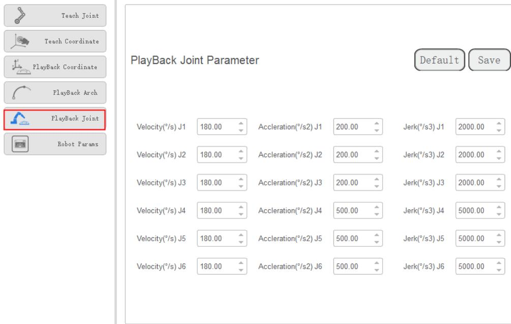
Figure 3.16 Playback parameters in the Joint coordinate system
