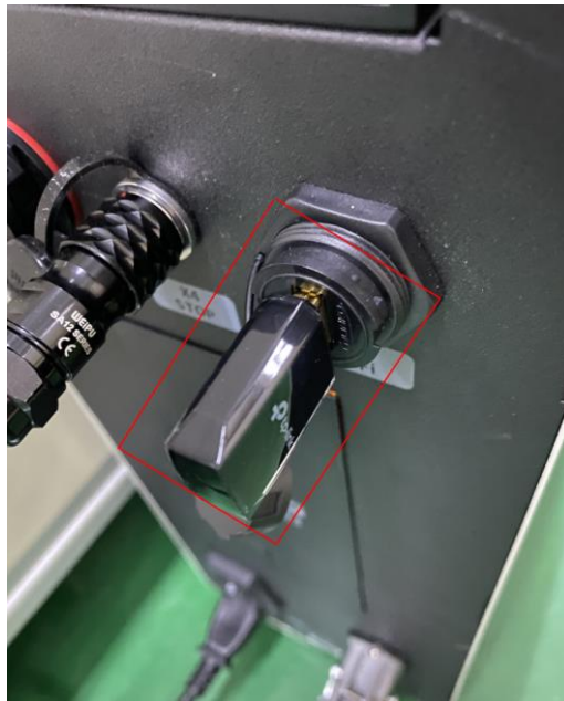
Figure 4.5 Connecting WiFi module
