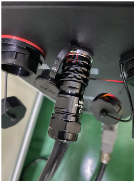
Figure 4.4 Connecting emergency stop switch
