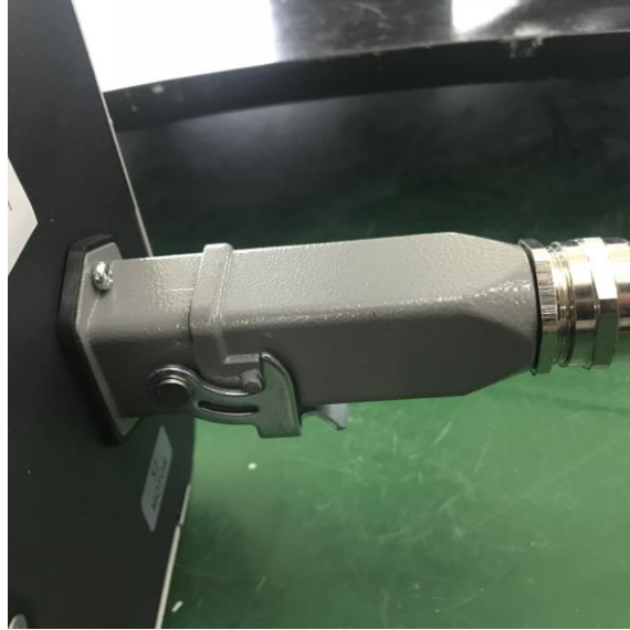
Figure 4.3 Connect controller and robot by heavy-duty cables
