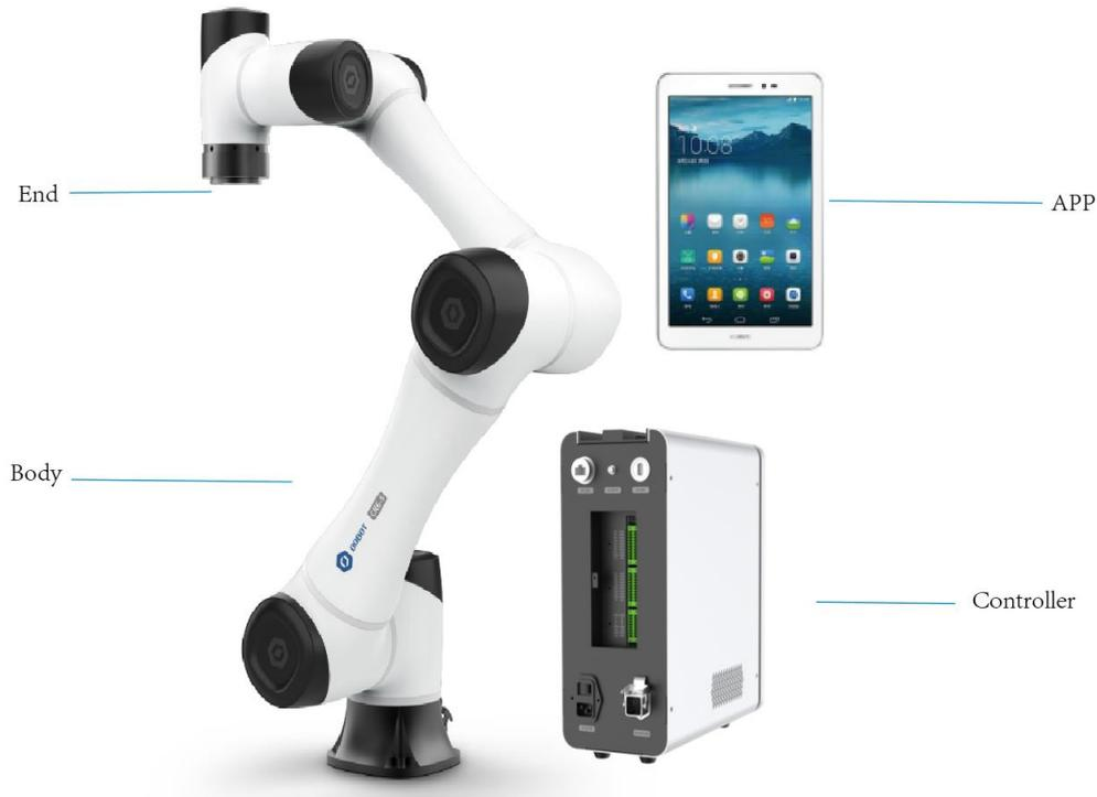
Figure 2.1 Robot system
