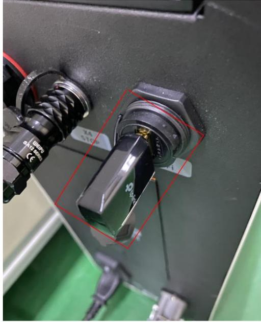
Figure 4.4 Connecting WiFi module
