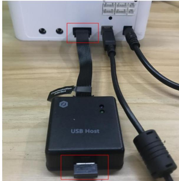
Figure 5.138 Connect with USB Host module
