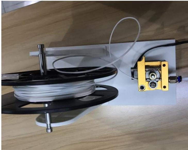
Figure 5.82 Place filament and extruder to the Filament holder
