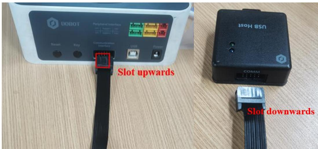
Figure 5.139 Connect Magician to USB host
