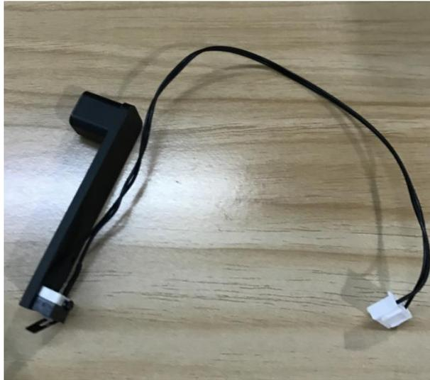
Figure 5.128 Auto-levelling tool
