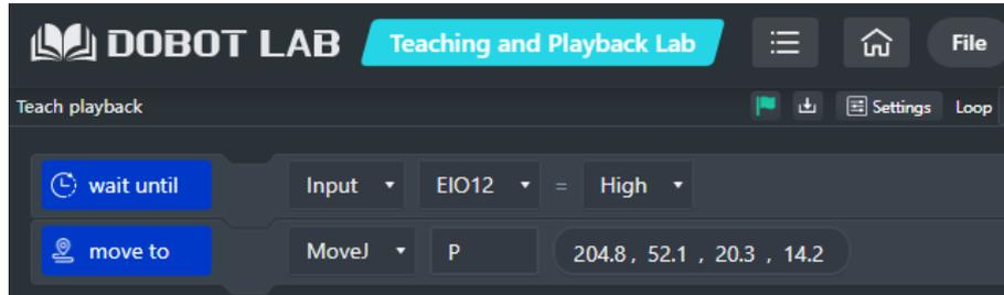
Figure 5.149 Move the trigger command
