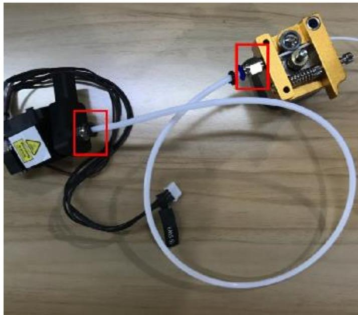
Figure 5.78 Connect extruder and hot end
