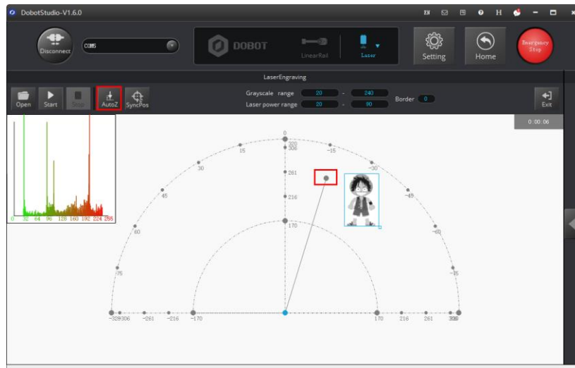
Figure 5.101 Lock the height of engraving
