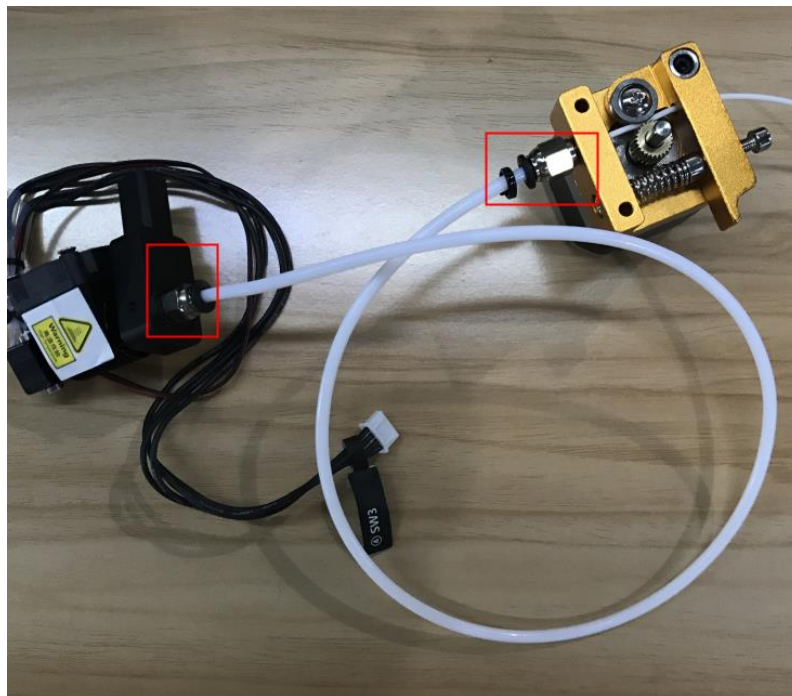
Figure 5.119 Connect extruder and hot end
