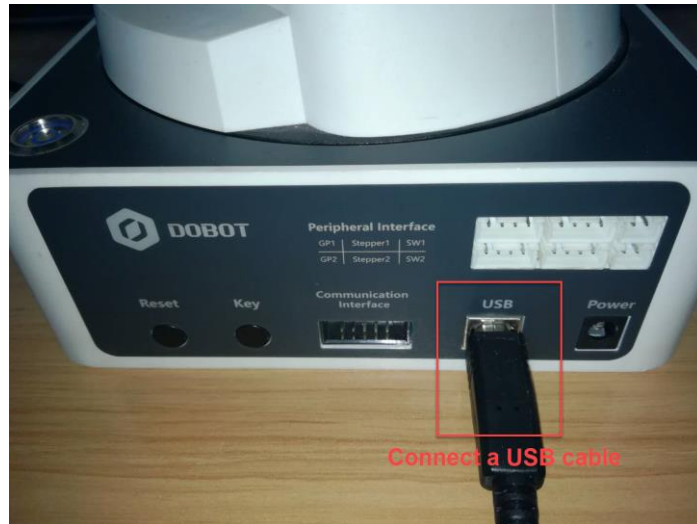
Figure 2.2 Connect the Dobot Magician to your computer
