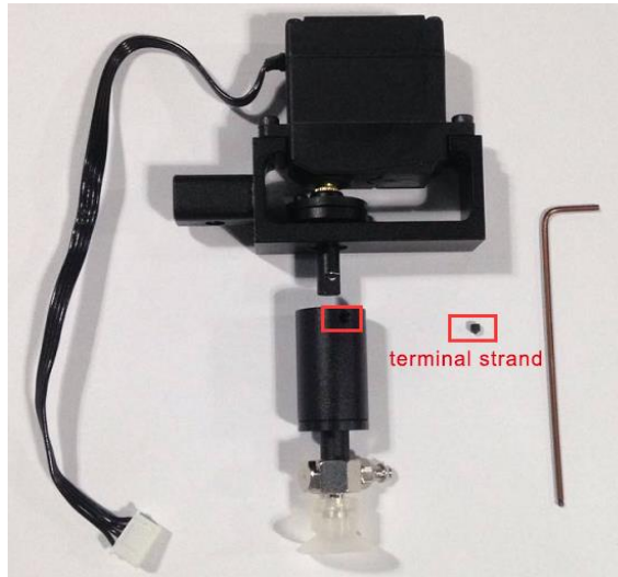
Figure 5.12 Dismantle the suction cup
