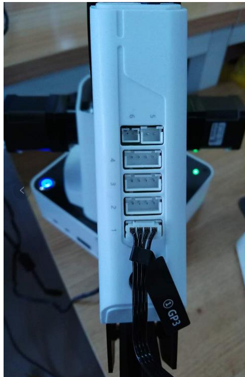
Figure 5.169 Insert the cable of the auto-levelling
