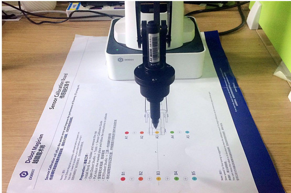
1. Figure 9.1 Put dobot in the marked place
