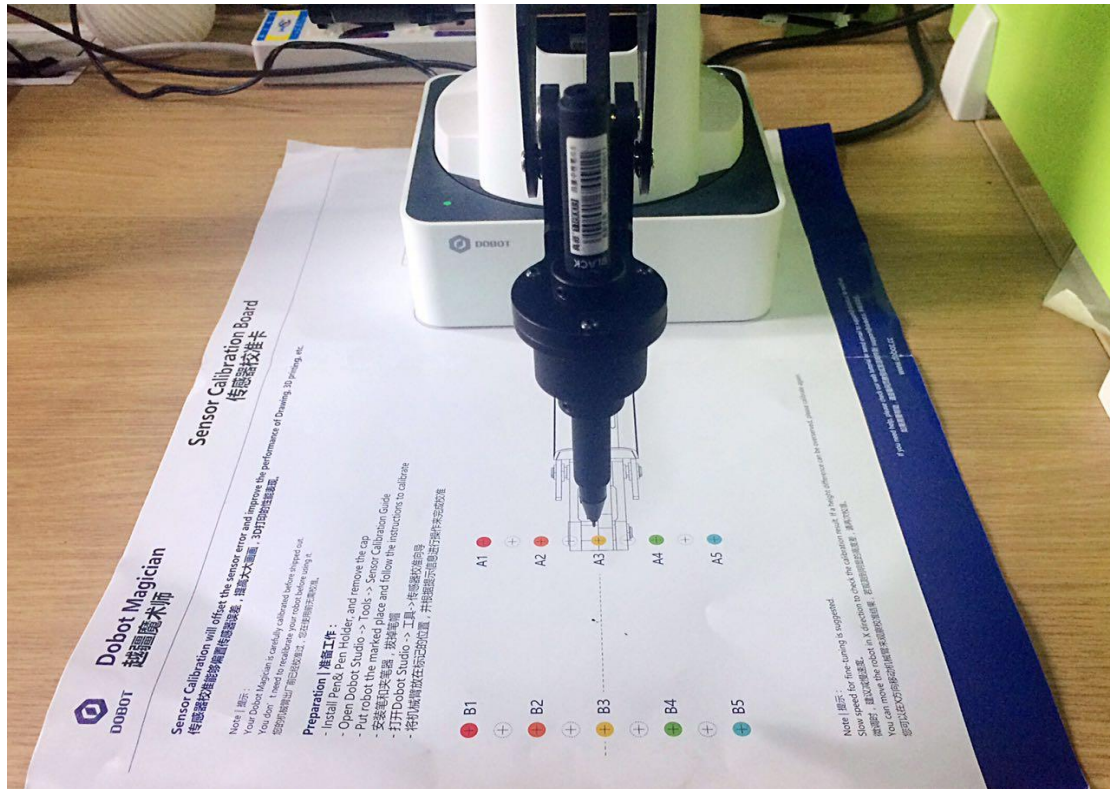
Figure 9.4 Put dobot in the marked place
